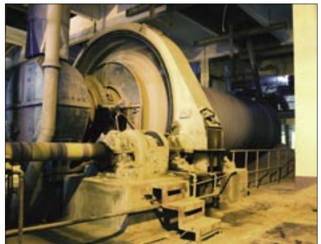
One of the old cement mills in operation
