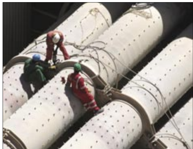
Maintenance of cooler tubes on one of the old kilns
