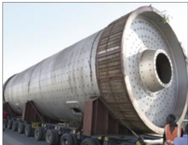
Transport of the new cement mill from port to factory
